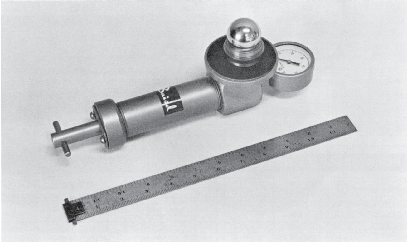
The Baird portable ball and seat tester is a light, hand operated tool designed to permit testing pump valves at the well location, or anywhere it is impractical to use our larger motor driven tester. To operate, place moistened ball and seat directly over the suction port in the rubber pad. Then actuate pump handle until desired pressure
